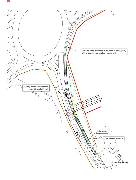
5.1 The proposed access point has been drawn up in detail here by Jubb engineers to demonstrate the technical feasibility of the proposed access, including achieving appropriate visibility in this location. It also indicates how the existing footpath network in the area could be improved and enhanced.
