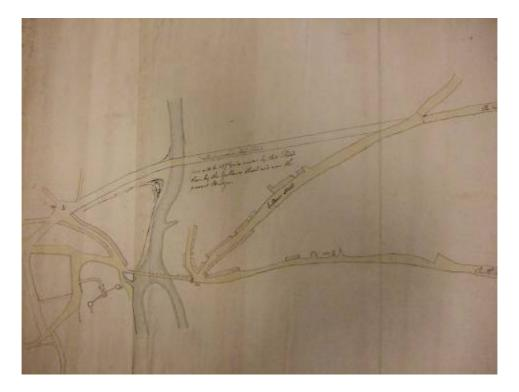
Fig 4.7: Plan showing proposed layout of new bridge and road, with old bridge crossing the Avon still in place (WCRO 1886 M278)
