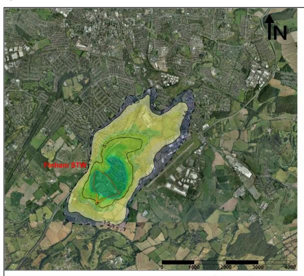
Contours of the areas are presented in which odour concentrations of 1.5 ou<sub>E</sub>/m³ and 5 ou<sub>E</sub>/m³ are exceeded for more than 175 hours per year for the current baseline (solid lines and green/yellow shading) and proposed digested sludge scheme (dashed lines and grey shading)
